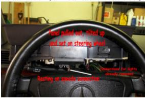
In this position you can disconnect the remaining wires on the right side, etc., especially the warning lamps I mentioned above.
