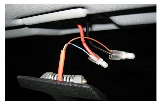
You can now re-install the mirror. Make sure none of the wires get pinched while putting the mirror back in. Also make sure the mirror wires and protective sheath looks like shown here
