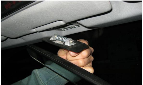
Remove the aluminium mount and mini sun visor
