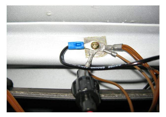
You can now re-install the aluminium mirror mounting bracket. Make sure it does not pinch the power/ground wires.
