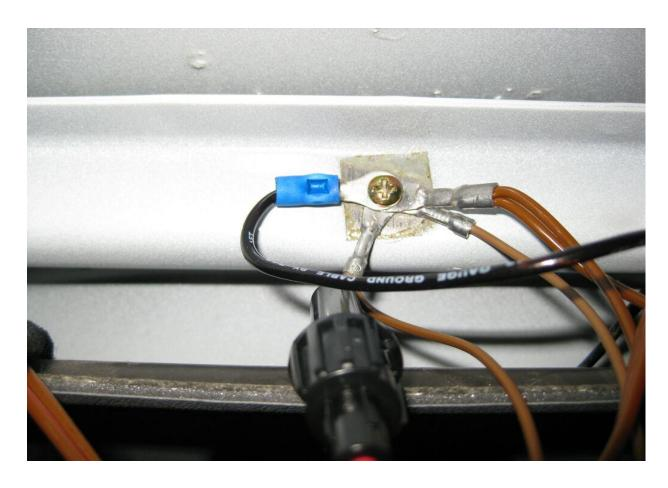
You can now re-install the aluminium mirror mounting bracket. Make sure it does not pinch the power/ground wires.
