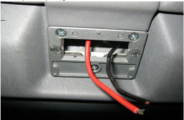
You can now spice the power/ground wires onto the mirror using the supplied crimp caps. This is where an extra set of hands comes in handy. Remember; only hold the mirror by the stalk! \* Your mirror will have red/black wires with red being the switched 12 volt and black being the ground \*
