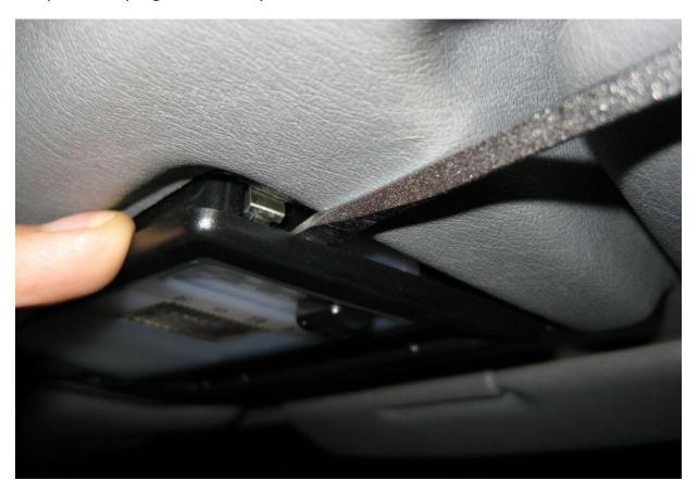
Unplug the 6 pin connector. On the 300ce the switched 12 volt is the black w/yellow stripe, but here you would verify this by using your multi-meter. This wire should have 12 volts with the vehicle ignition turned on, with the ignition turned off, there should be no power. DO NOT connect the mirror to a constant 12 volt power source.
