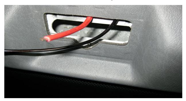
Going back to the black w/yellow striped wire, we cut it and use the crimp caps to splice in the red fuse wire like shown. Make sure the other end does not touch metal, as I ship the fuse holder with the fuse installed.
