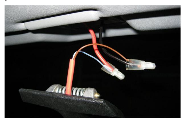
You can now re-install the mirror. Make sure none of the wires get pinched while putting the mirror back in. Also make sure the mirror wires and protective sheath looks like shown here
