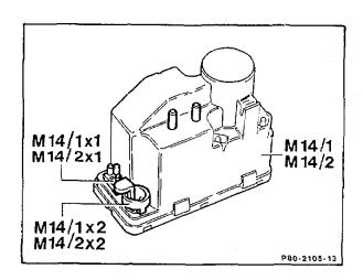
The actuators pass a negative control voltage during locking and a positive control voltage during unlocking through the connector (M14/1x2) to the supply pump.
