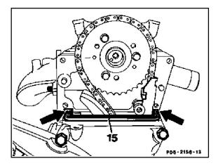
7 Fit insertion sleeve (arrow) 103 589 00 14 00 (for camshaft inner  $\varnothing$  21.6 mm), or 103 589 01 14 ( $\varnothing$  20 mm) onto the camshaft. Coat the sealing lip of the radial seal (14a) with engine oil. Fit on front cover (14).
