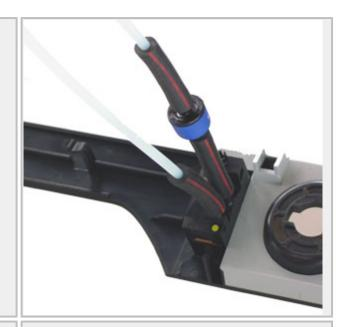
Reinstall the connectors and the speedometer cable behind the instrument cluster, and slide it back into place.
