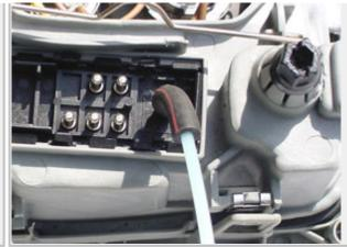
Pull up the floor mat behind the brake pedal, and unclip the speedometer cable clamp so it can move. Slip the wire hooks in on each side of the cluster, and ease it part way out, right side first.
